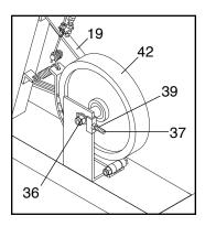
tighten the M8 Flanged Hex Nuts (36). Reattach the side shields.
